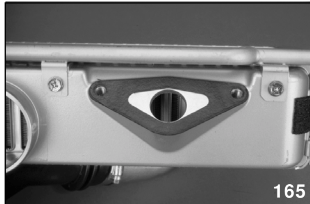
By-pass Valve Connection
