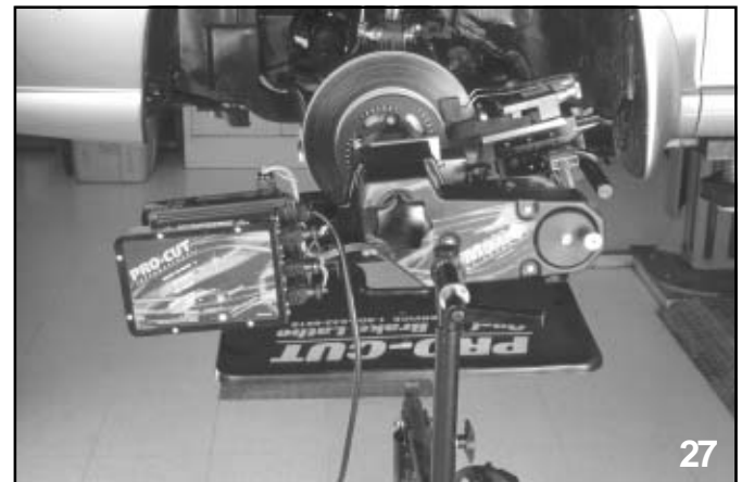
Rotor resurfacing
