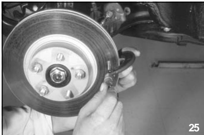
Measuring rotor thickness
