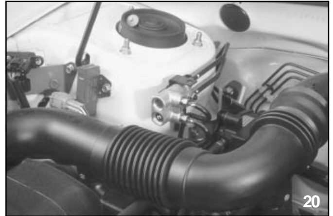
Typical proportioning valve
