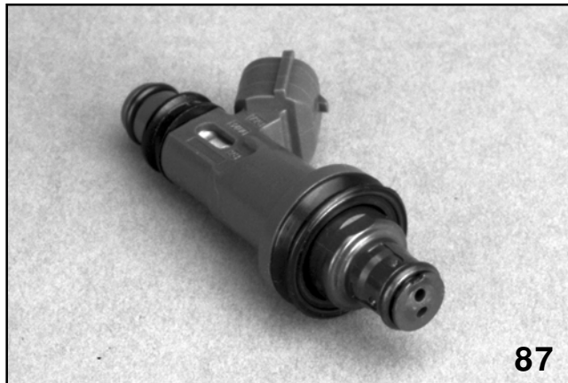
Air Assist Injector
