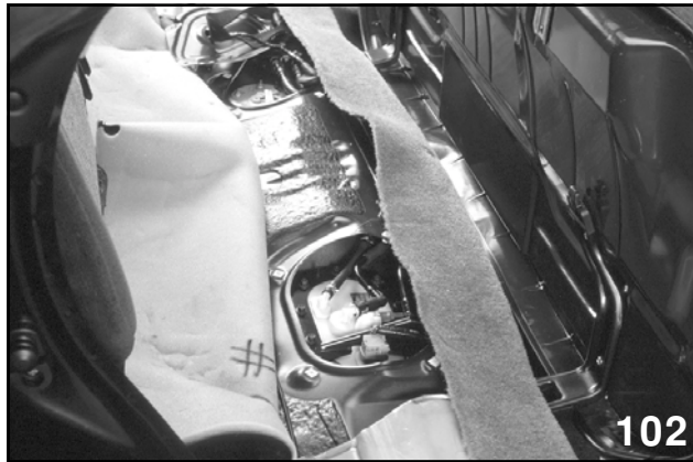
Fuel Pump (Under Seat)
