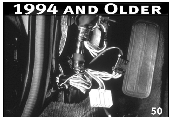
Select Monitor and Service Connector
