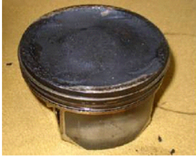
Ring Land Damage from Detonation
