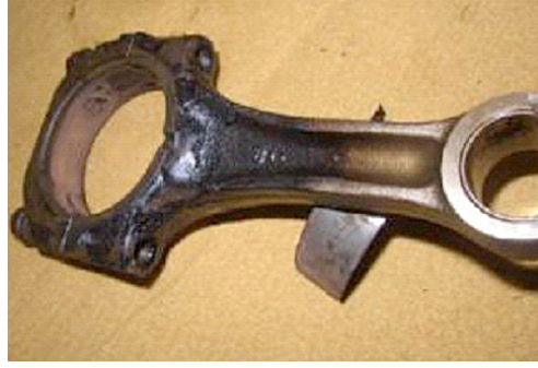
Rod Bearing Spun from Lack of Oil
