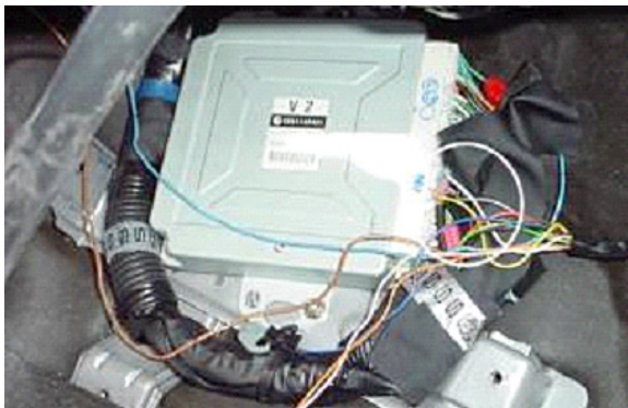
Aftermarket Air Fuel Controller wired to ECM
